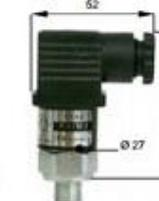
"F4" adjustable pressure switches allow a micro switch commutation once a preset pressure value is reached. The set point is adjusted working on the central screw (P3 execution) or intercepting the regulation screw situated inside the instrument, via a 2mm hexagonal key (M2 and M3). Rotating clockwise the set point is increased and vice-versa is decrease. Mechanical stops protect both the spring and the micro-switch from over pressurization.
